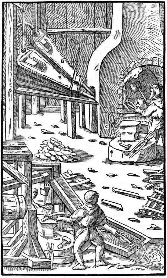
A-Forge. B-Bellows. C-Tongs. D-Hammer. E-Cold stream.
